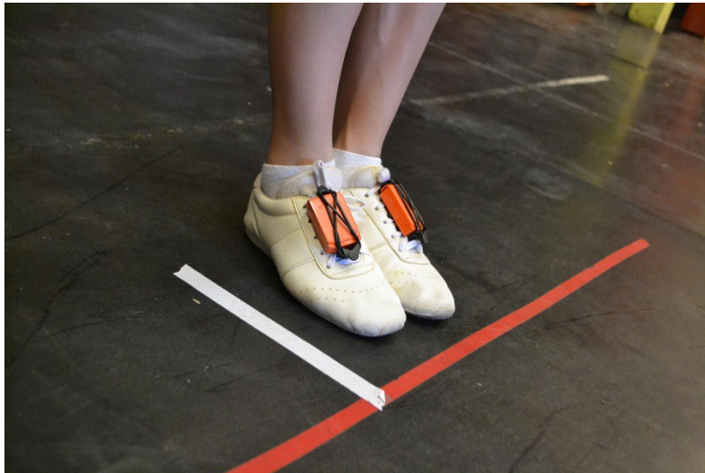
Fig. 2. Positioning of inertial sensors
